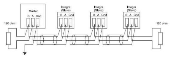
There must be no more than two wires connected to each terminal, this ensures that a "Daisy Chain or "straight line" configuration is used. A "Star" or a network with "Stubs (Tees)" is not recommended as reflections within the cable may result in data corruption.
