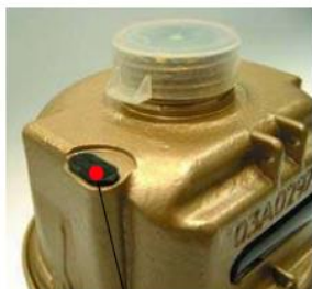
'A' Probe location position under protective plug.
