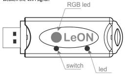
Connect LeON to a 5 volt USB power supply (not included). The LED will light up constantly at first, and flash continuously after 3 seconds. This means that the LeON is not yet connected to your WiFi network. Pairing with WiFi can ONLY be done manually, not via the server scanner or not via the app.
