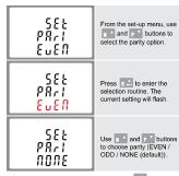
On completion of the entry procedure, press B to confirm the setting and press 4/1 to return to the main set up menu.
