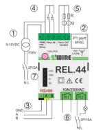
**Power supply:** [1] First connect the 12 Volt DC (Max. 2A, max. 2.5 meters and 2x0.5mm<sup>2</sup> with solid core), or power supply from MEMo3 (single + terminal) and then [2] P1 port input with RJ12 cable (max. 3 meters).
