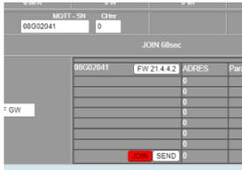
**Example MQTT:** Choose module type 'MQTT'. In the MQTT-SN box, enter the MAC address of the module to be linked (always 12
