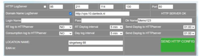
**Login Name - Pass:** In the HTTP server we must (for security reasons) also set up a user, password and possibly a folder where the data is stored.
