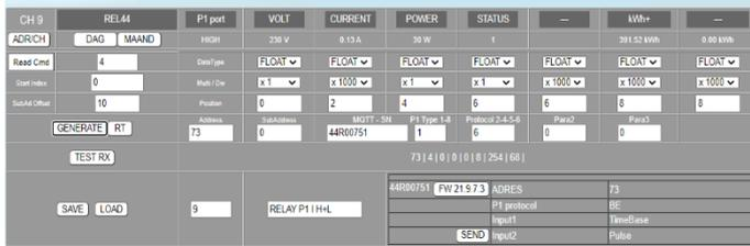
**Example REL44 OUT1-4:** according to the specs, the outputs start at index 90, and there is a shift of 1 between each output.
