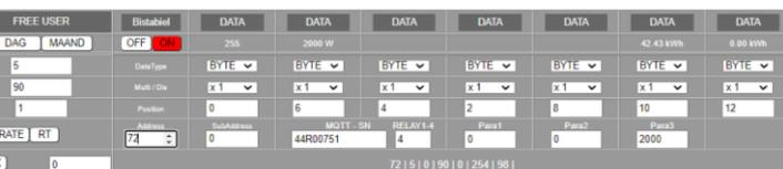
Press **'TEST TX'** to test this function. If the desired relay follows with the entered status, the OFF/ON buttons will also follow!
