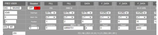
The input status (set to 255 here), now has only 1 data field because the selection is on BYTE.
