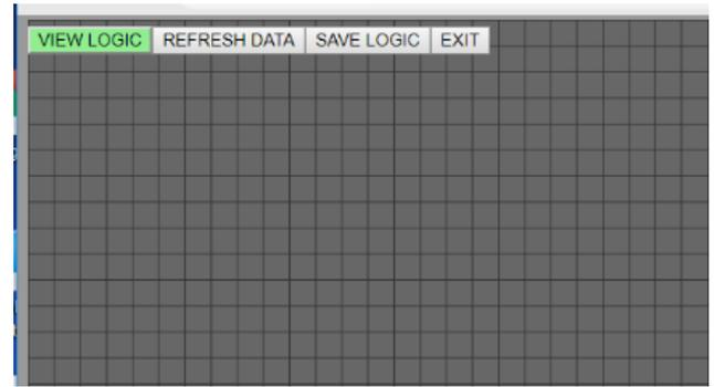
**VIEW LOGIC:** if this button lights up red, you have to wait a while for the logic to load. When the button lights up green, you can press this button. If logic has already been introduced, the logic will be shown. If no logic has been created yet, the screen remains blank.
