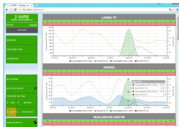
Clicking on **'OVERVIEW'** shows in a table a total overview of the electricity consumption, heating consumption (gas or oil), water consumption and possibly yield of solar panels.
