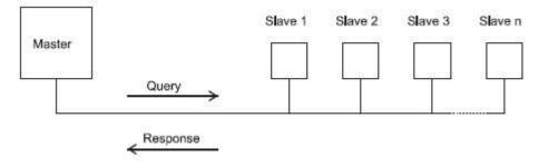
In the MODBUS Protocol the master can address individual slaves, or, using a special "Broadcast" address, can initiate a broadcast message to all slaves. The 2-WIRE Digital meter do not support the broadcast address.
